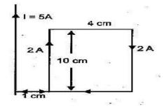
magnitude and direction of the loop due to the current carrying wire
